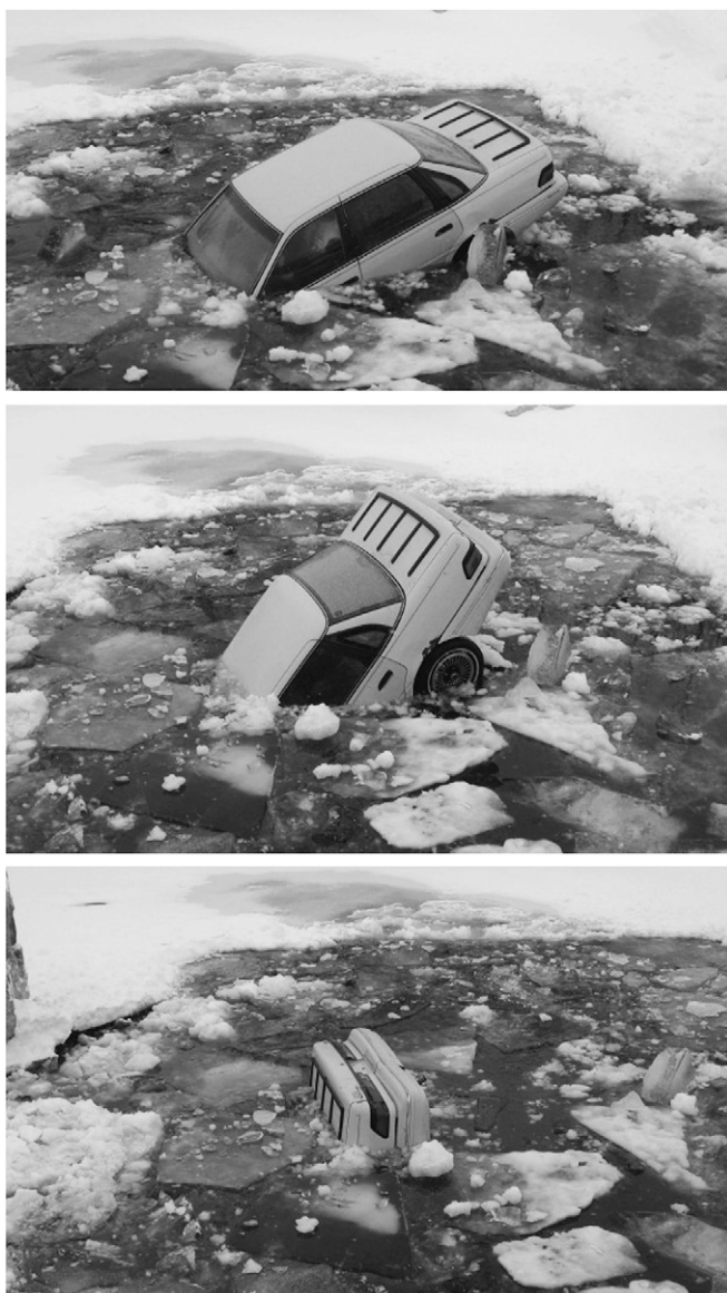
Fig. 2. Three phases of vehicle submersion: Top, floating; Middle, sinking; and Bottom, submerged (Manitoba, winter trial).
